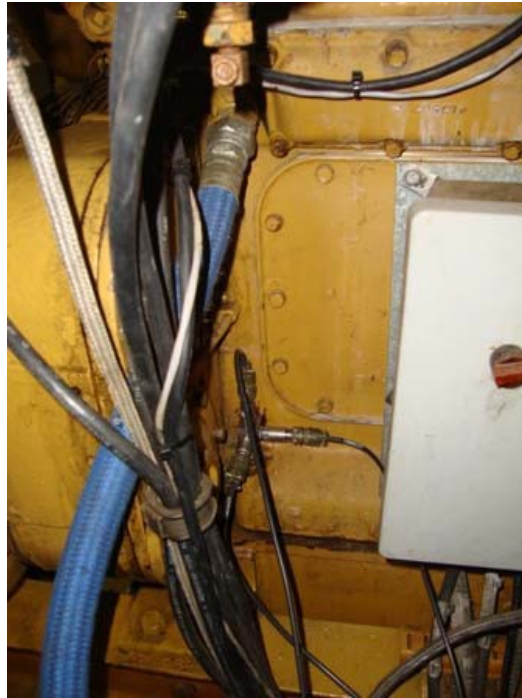
Figure 13. Diesel Engine Forward Accelerometers
