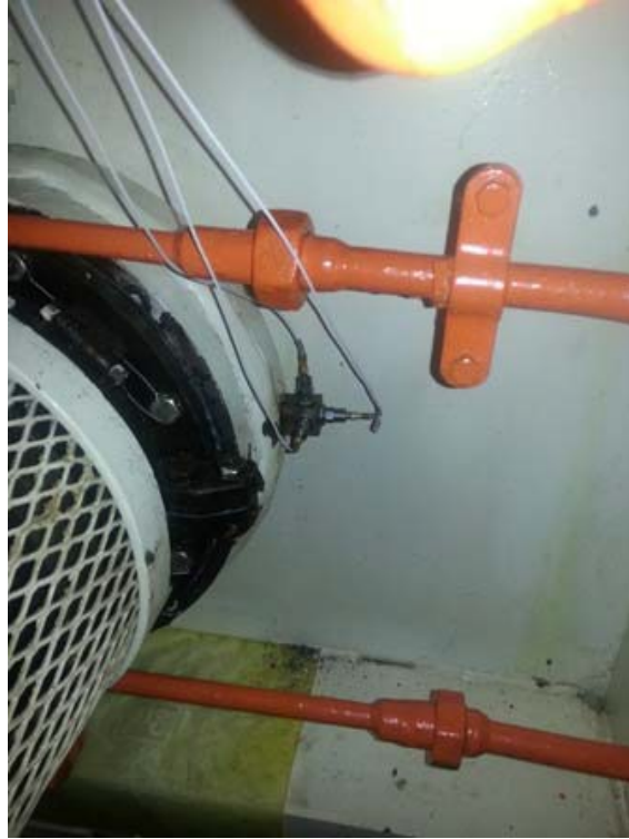
Figure 20. Propulsion Motor Lineshaft Bearing (By Shaft Seal) Accelerometer
