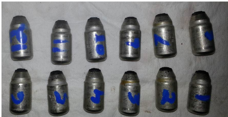
Figure 50. Post-Test Condition of Number 4 SSDG Nozzle Assemblies
