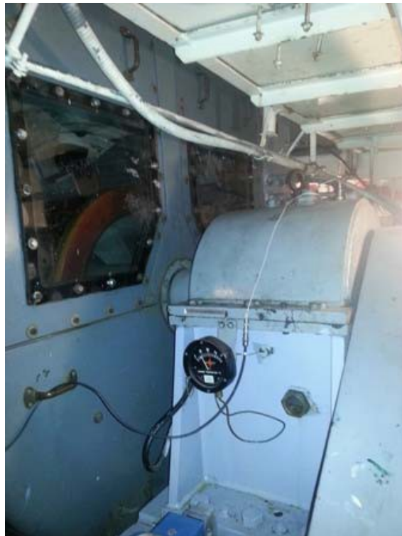
Figure 17. Propulsion Motor Journal Bearing Accelerometer
