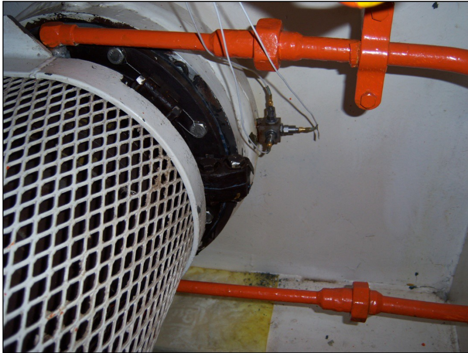
Shaft Seal (Stbd) Blocks facing inward for both shafts
