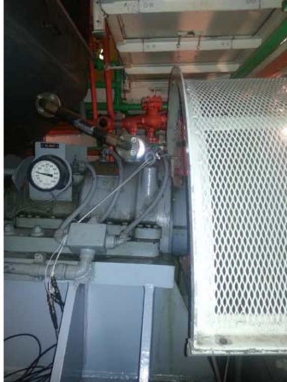
Figure 18. Propulsion Motor Thrust Bearing Accelerometers
