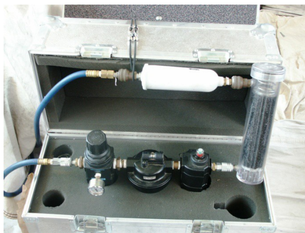
Figure B-2: Field Processing Unit for Purifying Dilution Air in Carrying Case
