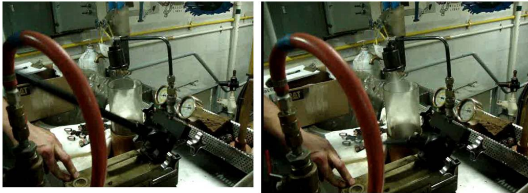
Figure 52. Nozzle Spray and Pressure Test – (spray/pop test shown at right)
