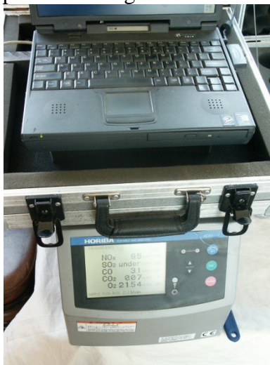
Figure B-3: Setup Showing Gas Analyzer with Computer for Continuous Data Logging
