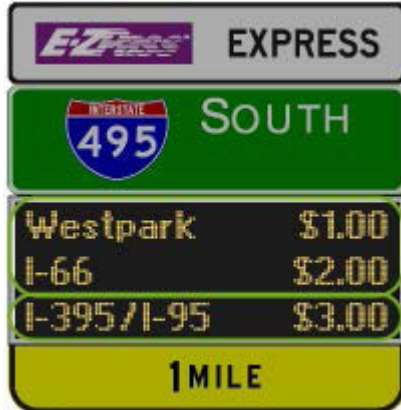
Figure 16. Dynamic Message Signs Used for Dynamic Tolling in the Metropolitan Washington Area 15
