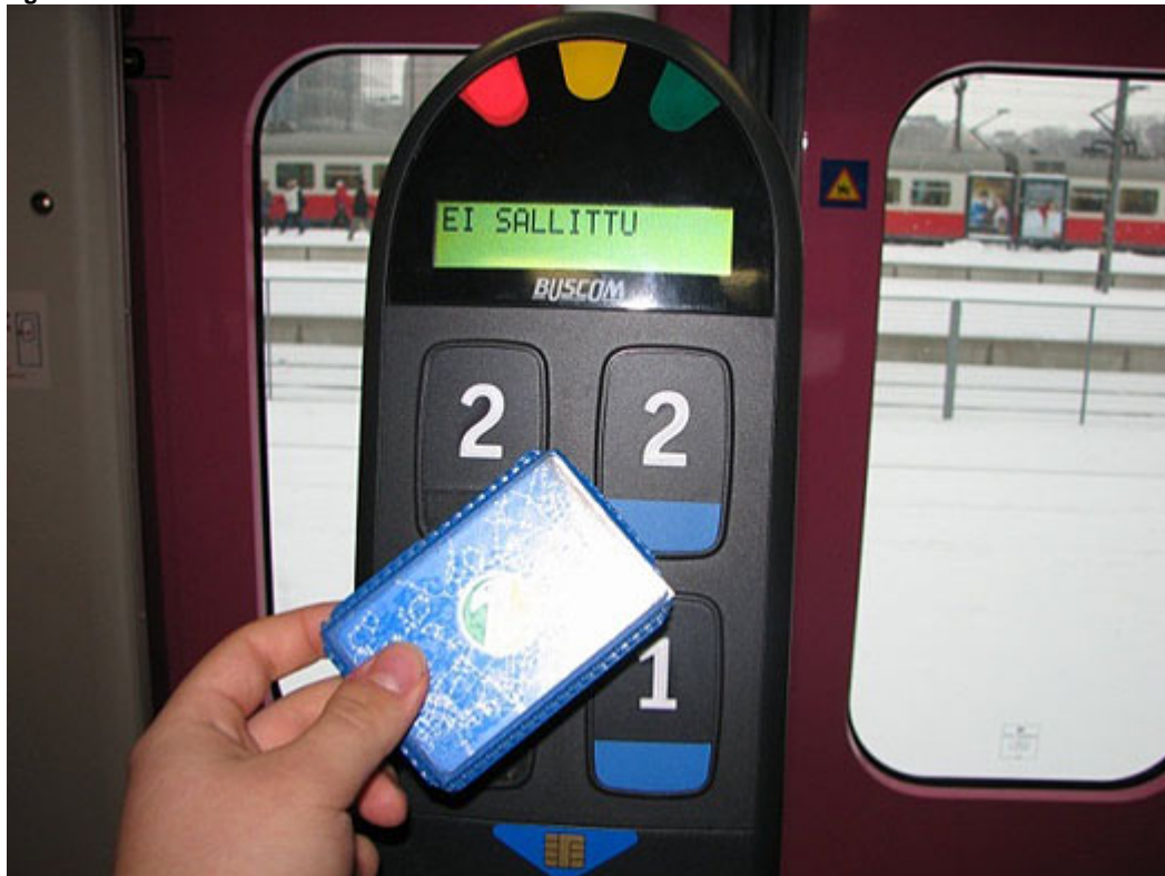
Figure 2. Contactless Smart Card in Use for Transit in Finland 4
