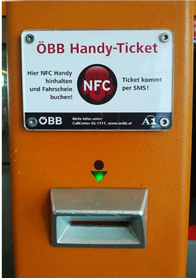
Figure 3. Example of a Ticket-Stamping Machine of the Austrian Federal Railways that Can Be Used to Purchase Mobile Tickets 6
