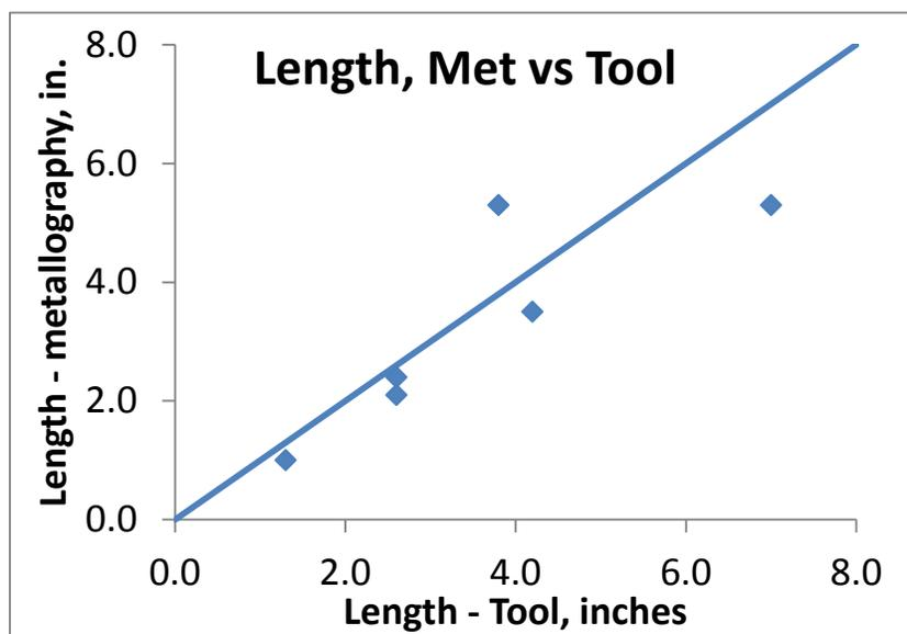
**Figure 54. Comparisons of Lengths Found by Metallography with Those Found by CMFL Tool**
