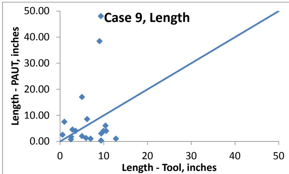
Figure 33. Comparisons of Lengths as Indicated by ILI and Those Found by Phased-Array UT
