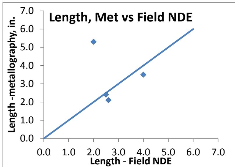
**Figure 56. Comparisons of Lengths Found by Metallography with Those Found by Field NDE**
