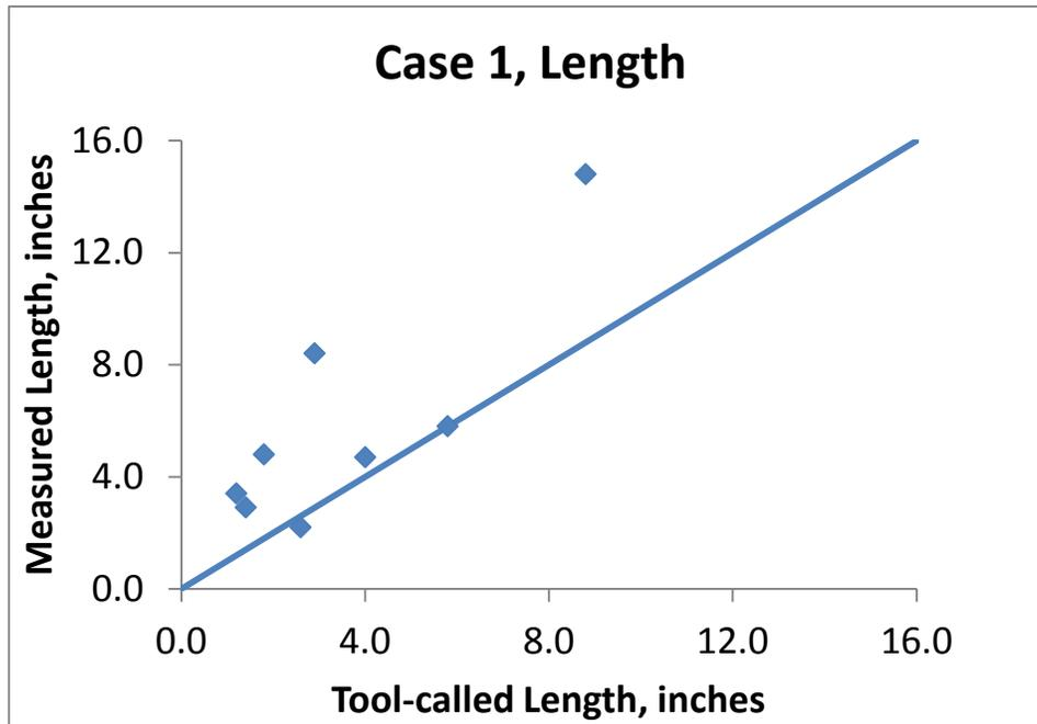
**Figure 2. Comparisons between Field-determined Anomaly Length and ILI Anomaly Length, Case 1**
