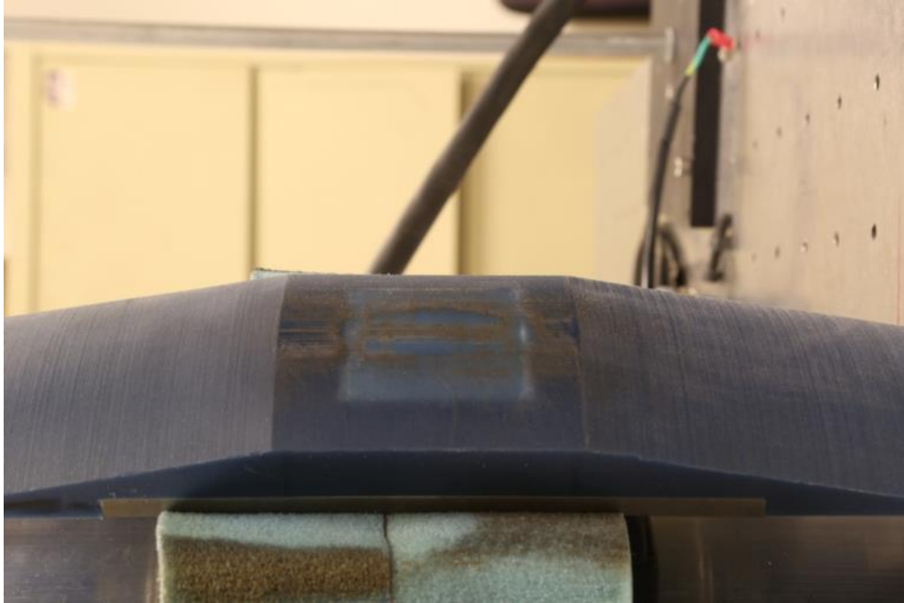
Figure 101. Side View of the Sensor Shoe after 1,439 meters of Axial Travel
