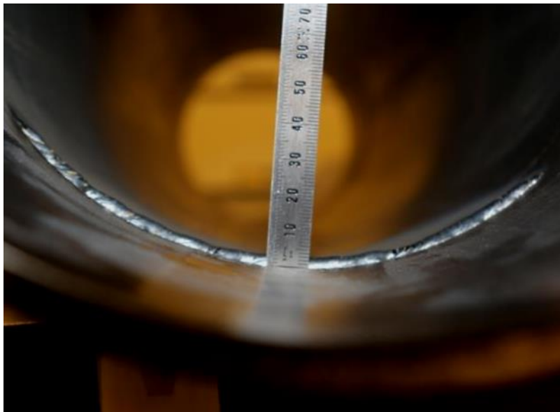
Figure 94. 3 mm Tall Bead Welded in the Seamed Pipe Sample
