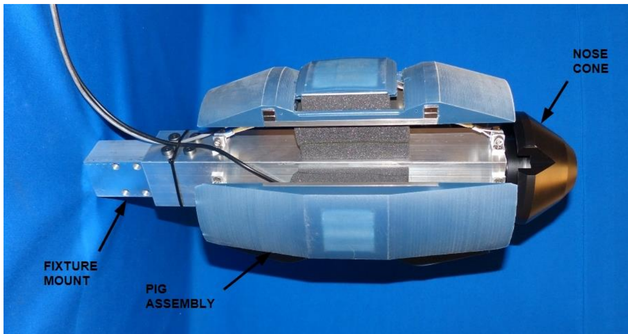
Figure 57. Completed Pig Assembly
