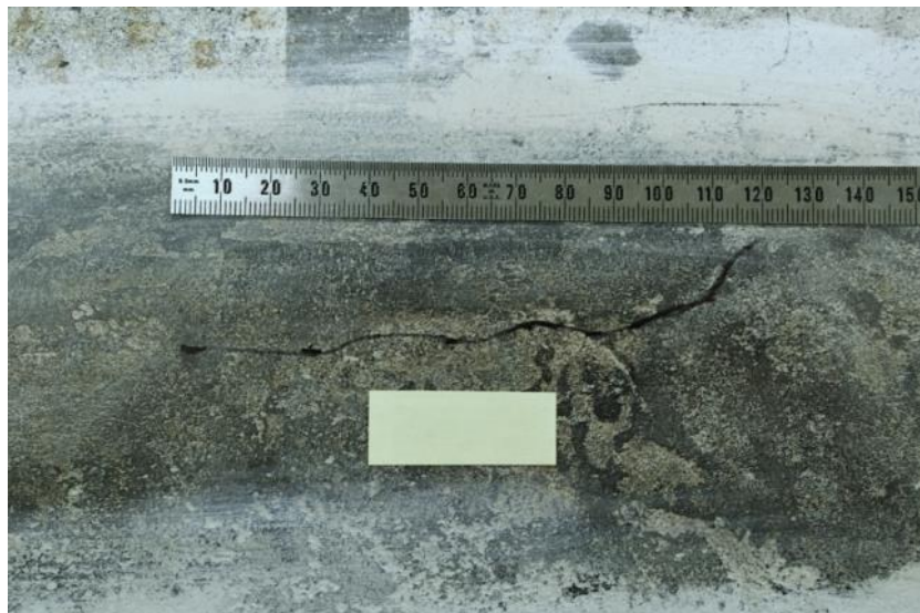
Figure 72. SCC Sample with the Approximate Crack Location Noted – OD View
