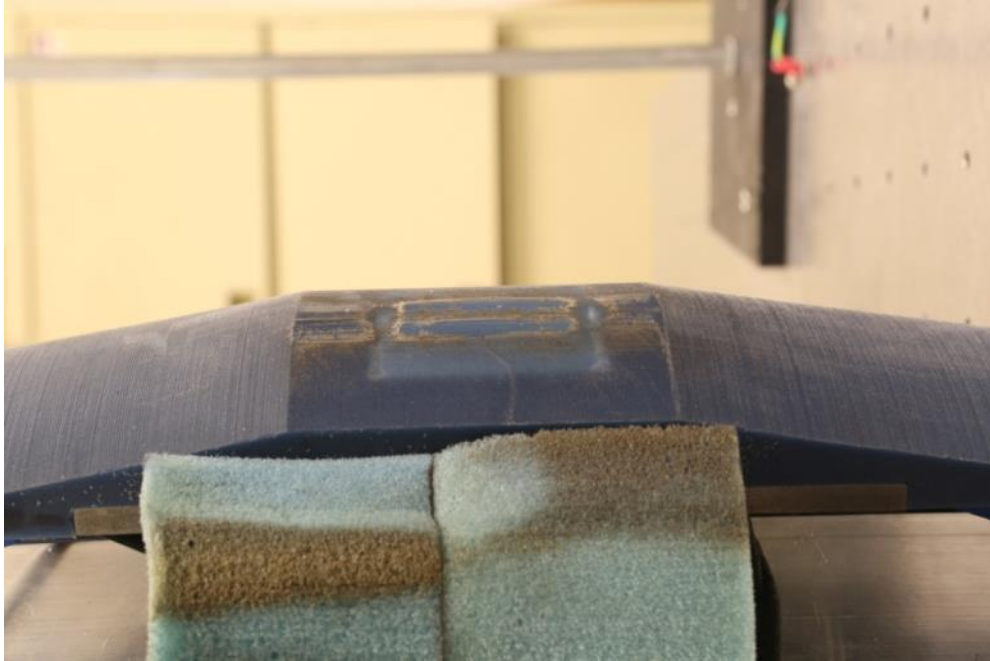
Figure 107. Side View of the Sensor Shoe after 4,933 meters of Axial Travel
