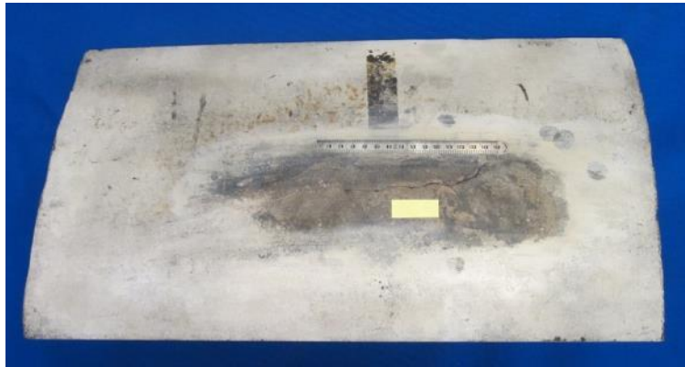
Figure 71. SCC Pipe Sample – OD View
