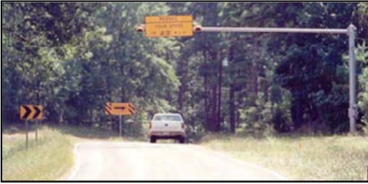
Figure 34. Photo. Texas System curve advisory speed limit sign. Camp County, Texas.
