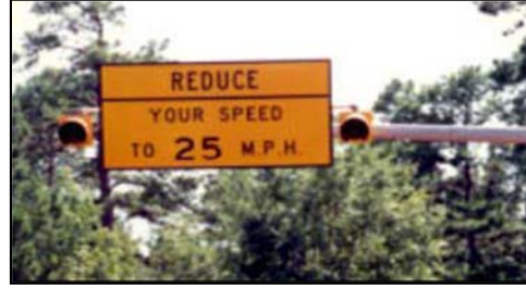
Figure 35. Photo. Texas System curve advisory speed limit sign. Camp County, Texas.
