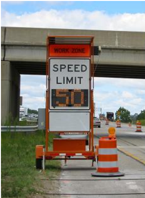
Figure 1. Variable speed limit system deployed in Michigan varied the speed limit based on nature of road work activity and traffic conditions.
