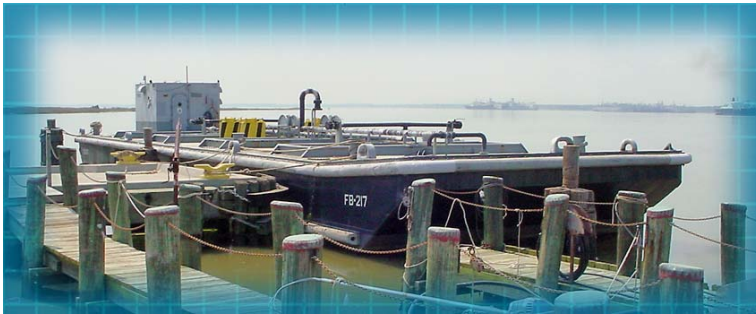
Ballast water testing platform being converted for testing technologies.
