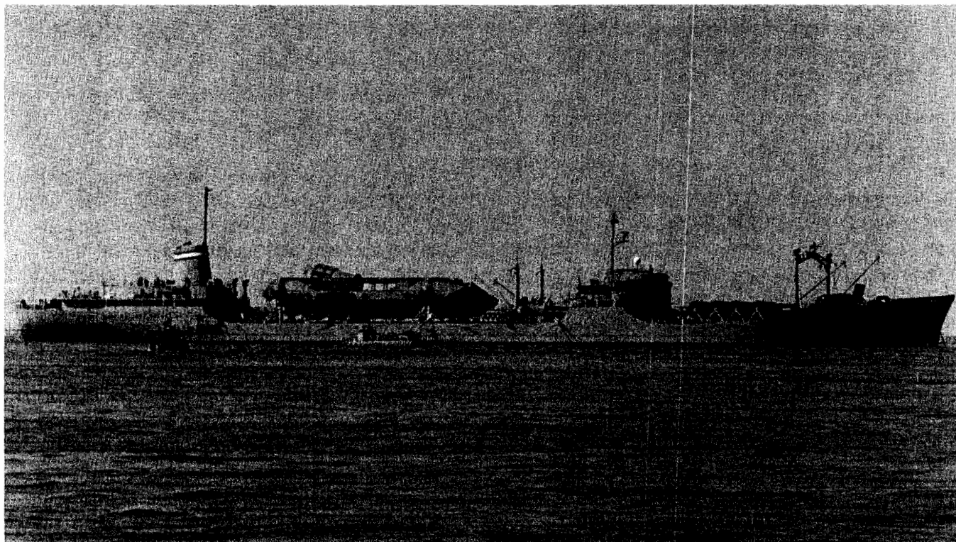
The OPDS Conversion Program uses modified tankers to supply fuel to Marine Corps and Army beach units from an offshore mooring. Conversion of the third, the SS CHESAPEAKE shown here, was completed during FY 1991.
