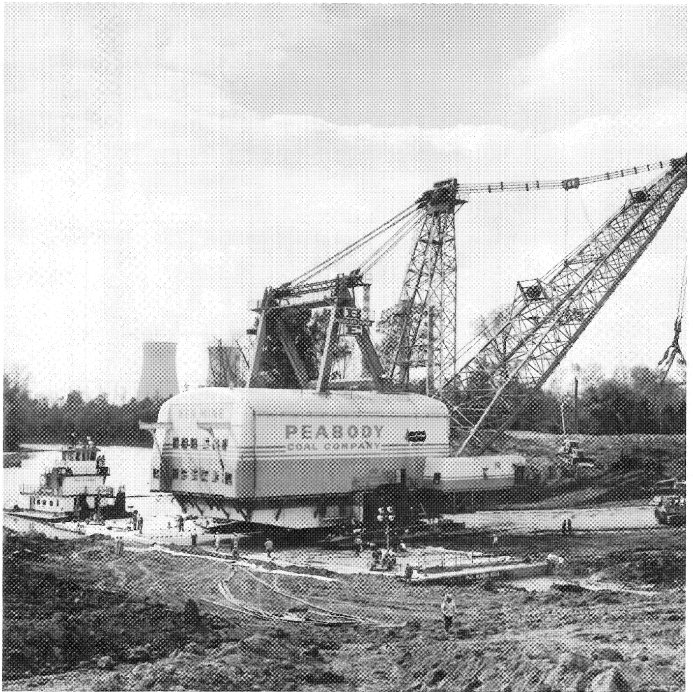
Believed to be the heaviest piece of equipment moved on the inland waterways, a 3,000-ton dragline crane is loaded aboard the heavy-duty deck barge PAUL BUNYON. A second barge supported the lowered boom, and two others were used to increase stability.
