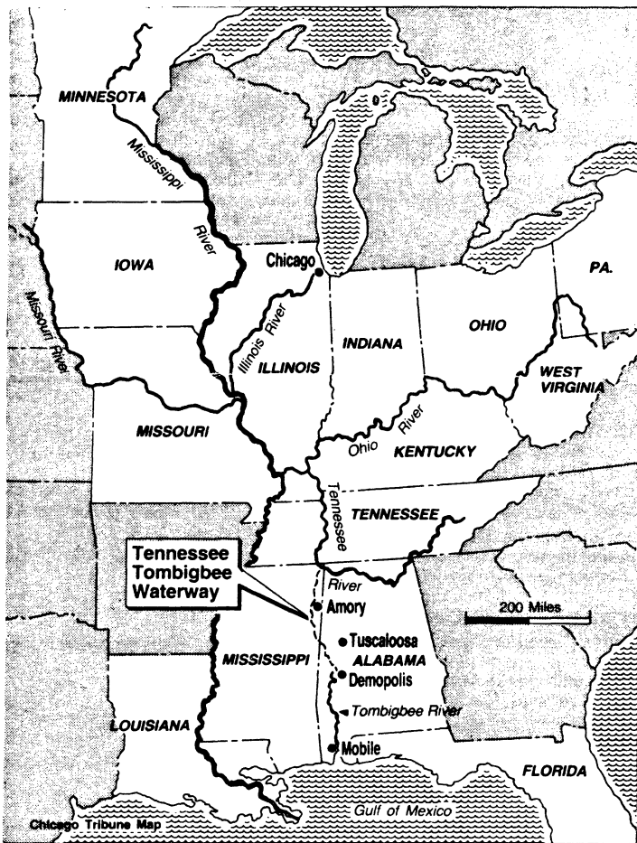
The first towboat and barges moving 7,700 tons of petroleum products from Mobile to Sheffield (AL) through the newly opened Tennessee-Tombigbee Waterway. The Tennessee-Tombigbee Waterway, opened on January 10, 1985, is the constructed link joining the Tennessee River with the Black Warrior-Tombigbee Waterway. The waterway incorporates 10 locks and 5 dams and provides total lift of 341 feet.
