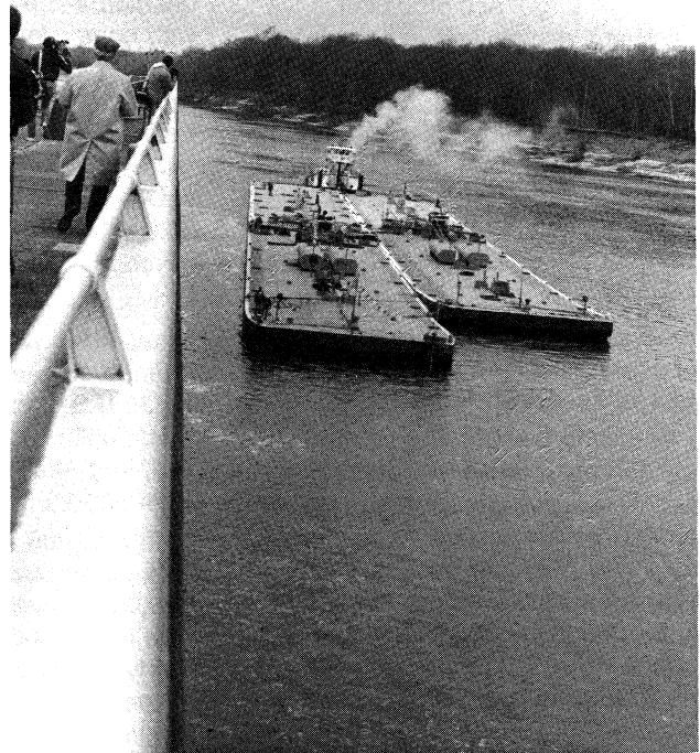
The first towboat and barges moving 7,700 tons of petroleum products from Mobile to Sheffield (AL) through the newly opened Tennessee-Tombigbee Waterway. The Tennessee-Tombigbee Waterway, opened on January 10, 1985, is the constructed link joining the Tennessee River with the Black Warrior-Tombigbee Waterway. The waterway incorporates 10 locks and 5 dams and provides total lift of 341 feet.
