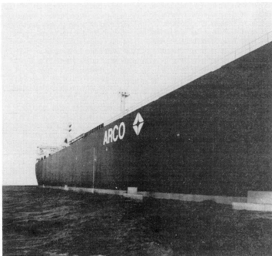
ARCO TEXAS, 70,000-deadweight-ton tanker operated in Alaskan oil trade, sea-tests use of copper-nickel sheathing to keep vessel's hull clean and free from corrosion. Note rectangular panels along water line. Research in corrosion-free hulls promotes energy efficiency in ship operations.
