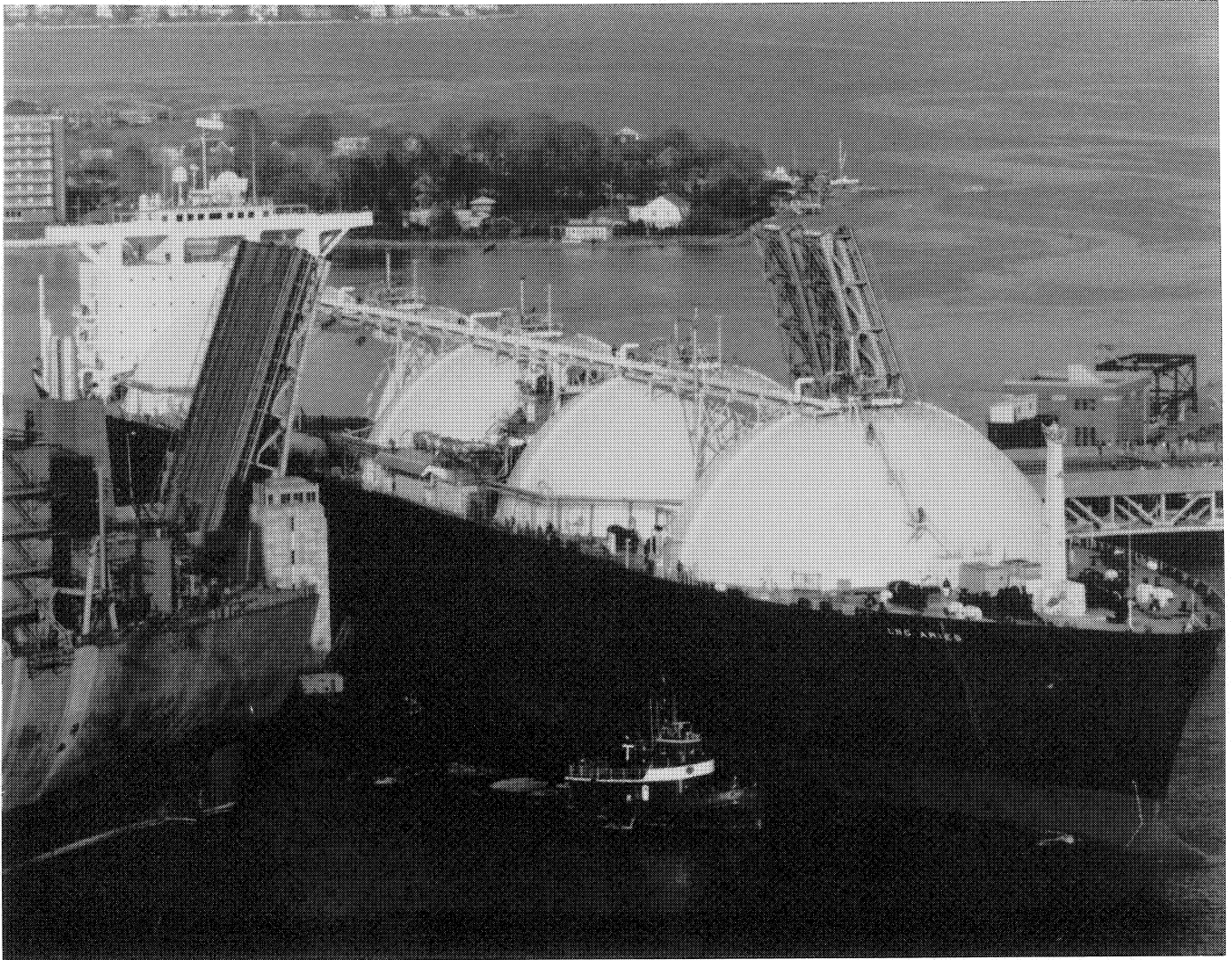
LNG ARIES, second liquefied natural gas carrier to be delivered by General Dynamics' Quincy (Mass.) Shipbuilding Division, squeezes through drawbridge after completing her sea trials. Huge ship, with capacity of 125,000 cubic meters, will be operated under U.S. flag, carrying LNG from Indonesia to Japan.
