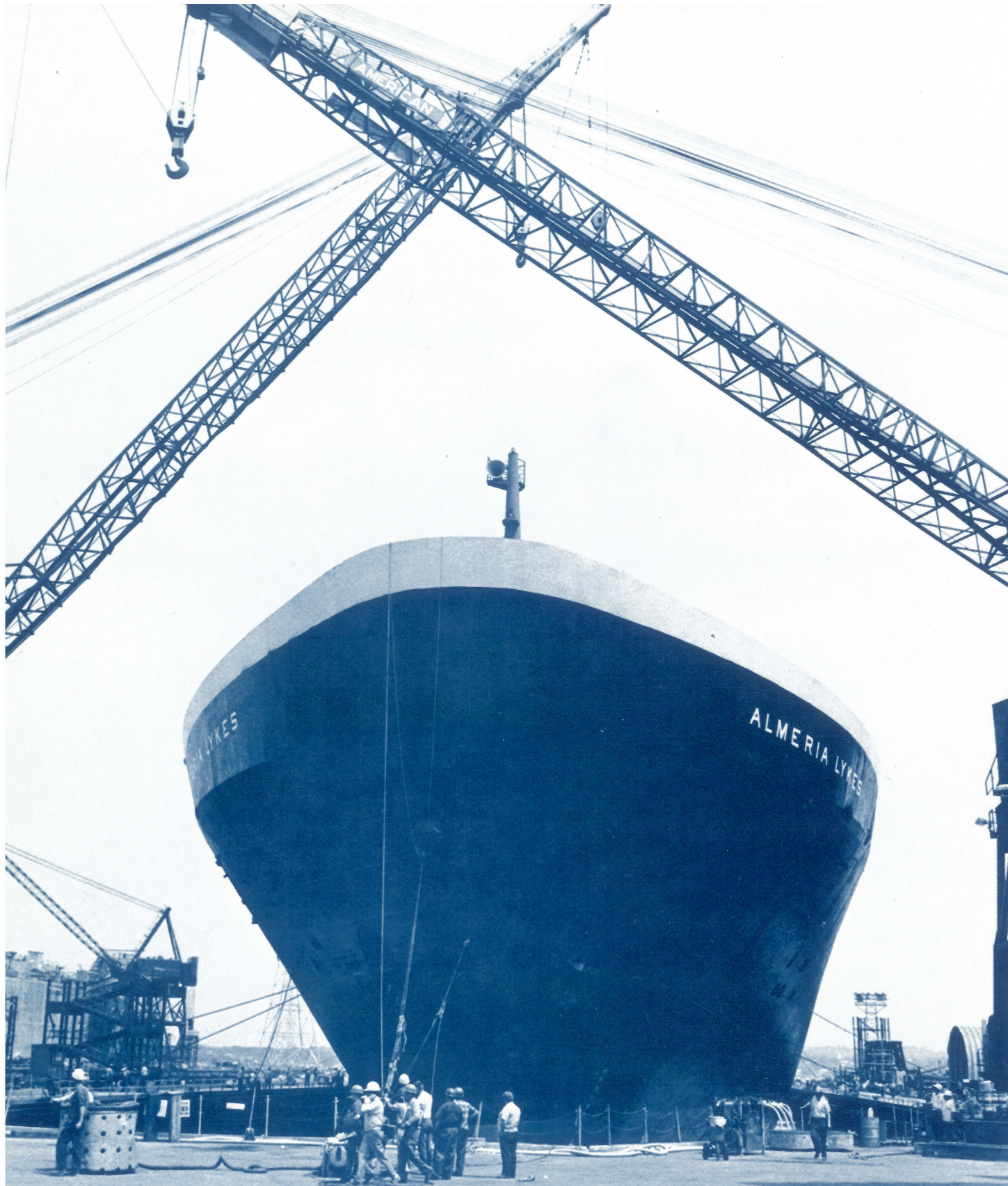
Employees at the Quincy, Mass., Shipbuilding Division of General Dynamics Corp. ready the SS ALMERIA LYKES for its sea trials. The huge barge-carrier is the second of three Seabee-class ships being constructed for Lykes Bros. Steamship Co., Inc.
