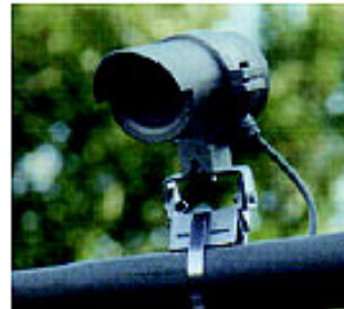
Siemens Eagle PIR-1 sensor. Performs vehicle counting, stop line presence detection, occupancy detection, and queue detection. (Photograph courtesy of Siemens ITS, Austin, TX).
