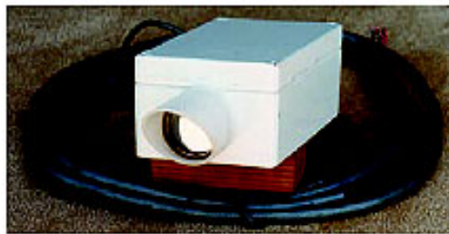
Eltec 842 passive infrared vehicle presence sensor. [Source: L.A. Klein, Sensor Technologies and Data Requirements for ITS (Norwood, MA: Artech House, 2001)].
