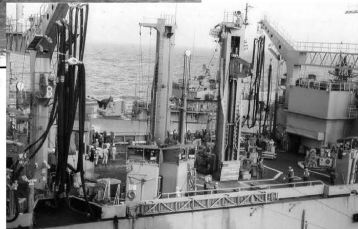
THE USS *WICHITA* WAS THE FIRST OF SEVEN SHIPS DESIGNED AS AUXILIARY REPLENISHMENT OILERS (AOR) THAT SERVED IN THE U.S. NAVY. THE NAVY BASED THE DESIGN OF THE *WICHITA* CLASS ON THE *SACRAMENTO* (AOE-1), WHICH WAS A FAST COMBAT SUPPORT SHIP. THE AOR WAS SLIGHTLY SMALLER, SLOWER, AND CARRIED LESS CARGO THAN AN AOE, BUT RETAINED THE SAME CONFIGURATION FOR TRANSFERRING SUPPLIES.
