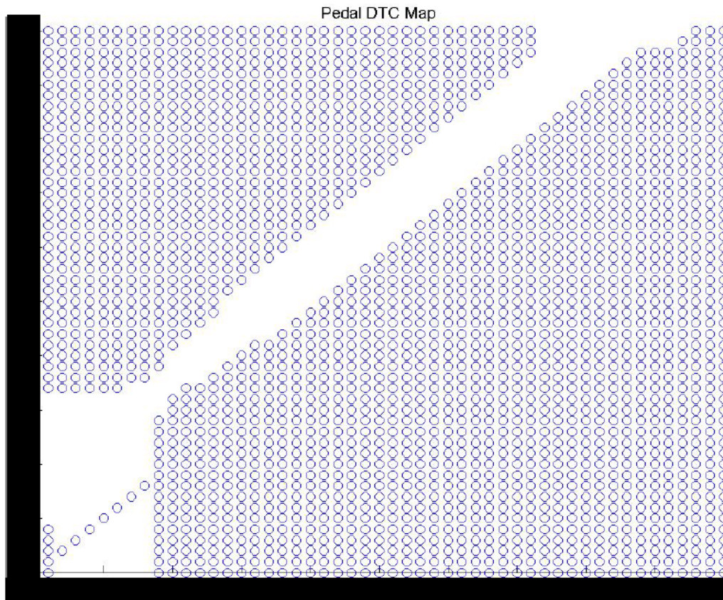
Figure A.11-7. Pedal Diagnostic Map for 2 second Ramp Sequence(Battery Voltage Applied)
