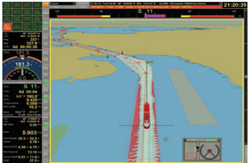
New 3D and Draft Optimizer equipment takes real-time ship's speed and position, the latest charting survey information, and performs complex calculations to provide a "safe look ahead" in shallow areas.
