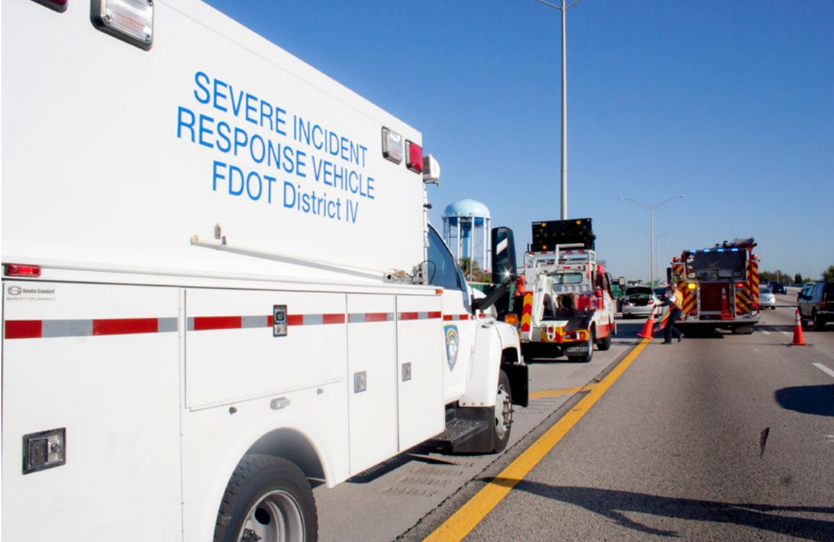
Figure 23. One of the design considerations for TIM is shoulder width for accommodating response vehicles. (Source: Florida Department of Transportation)
