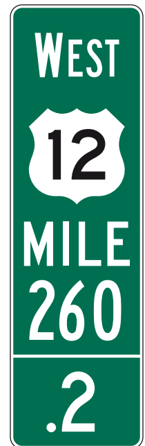
Figure 14. One-tenth mile markers support incident management on freeways. (Source: MUTCD)
