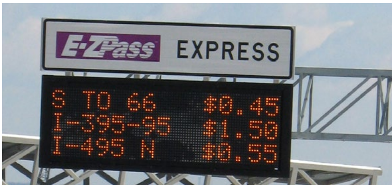
Figure 3. Express high occupancy/toll lanes with variable pricing is an M&O strategy increasingly used in the United States. (Source: SAIC)
