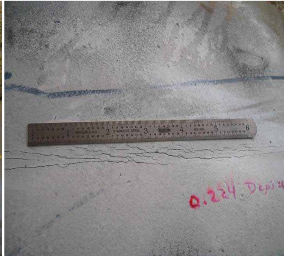
Top of Pipe Mechanical Damage/Gouge Multiple Dents
