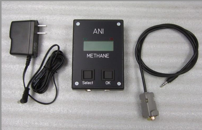
Analytical tool engineering prototype: Sensor kit includes DC power supply, software, sensor with built-in sensor head, and RS-232 cable
