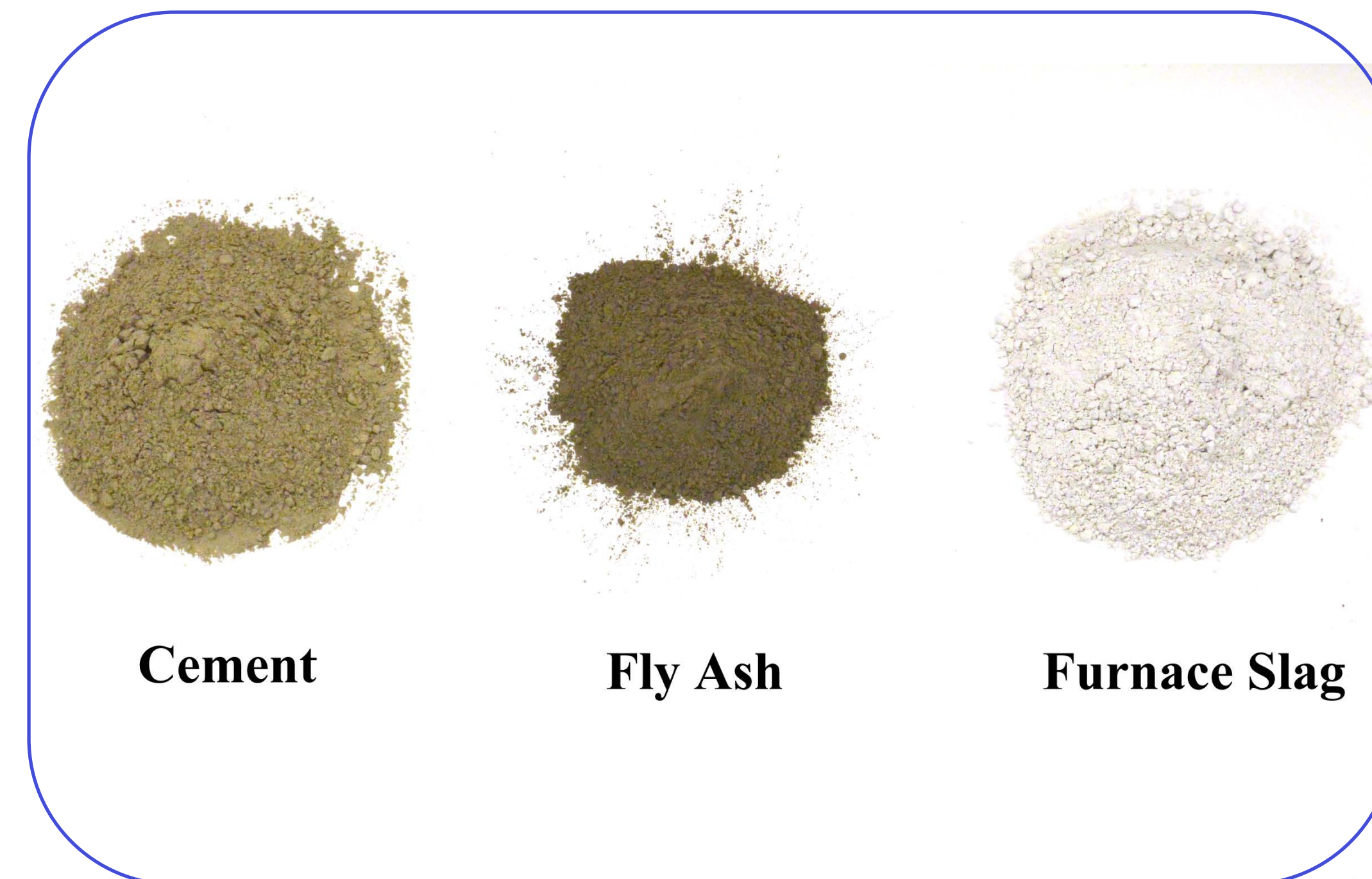
Figure 2. Supplementary cementitious materials
