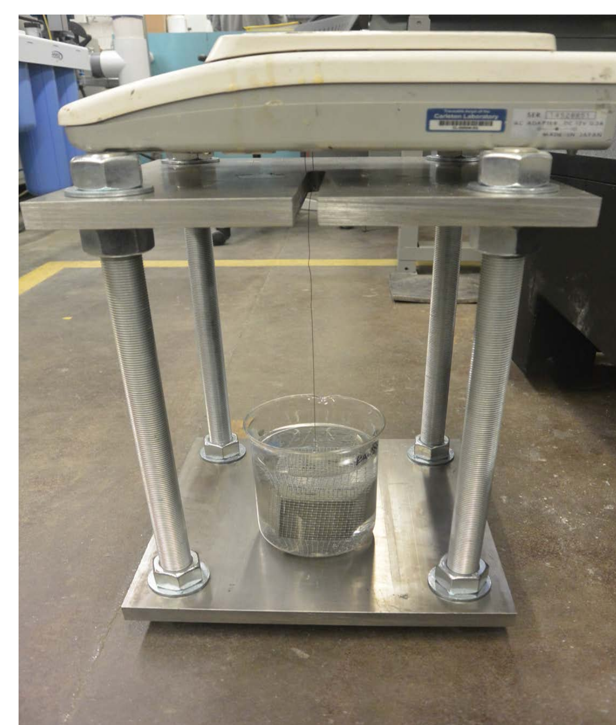
Figure 4. Test setup for measuring porosity
