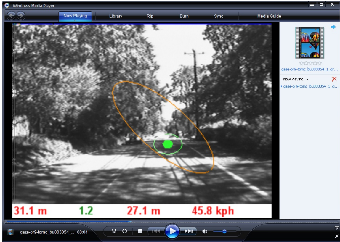
Figure 5. Reduced gaze video with sight distance information (Data from left to right: sight distance, sight distance to stopping distance ratio, stopping distance, motorcycle speed)
