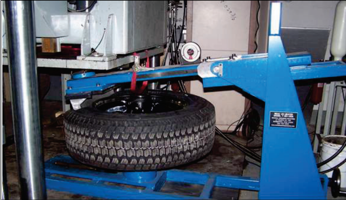
Figure 2.2. Bead Unseating Fixture at ARDL
