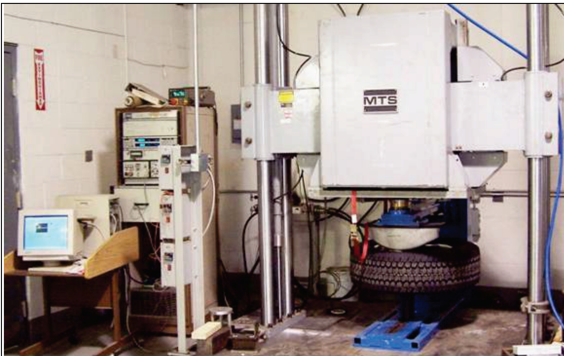
Figure 2.3. MTS Load Frame and Computer at ARDL
