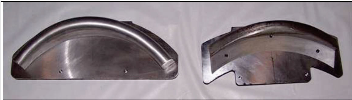
Figure 2.6. Bead Unseating Blocks BFNT 2B and ASTM 2B
