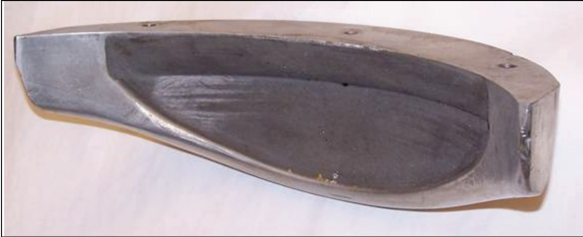
Figure 2.5. Bead Unseating Block Historical 2A (FMVSS No. 109)
