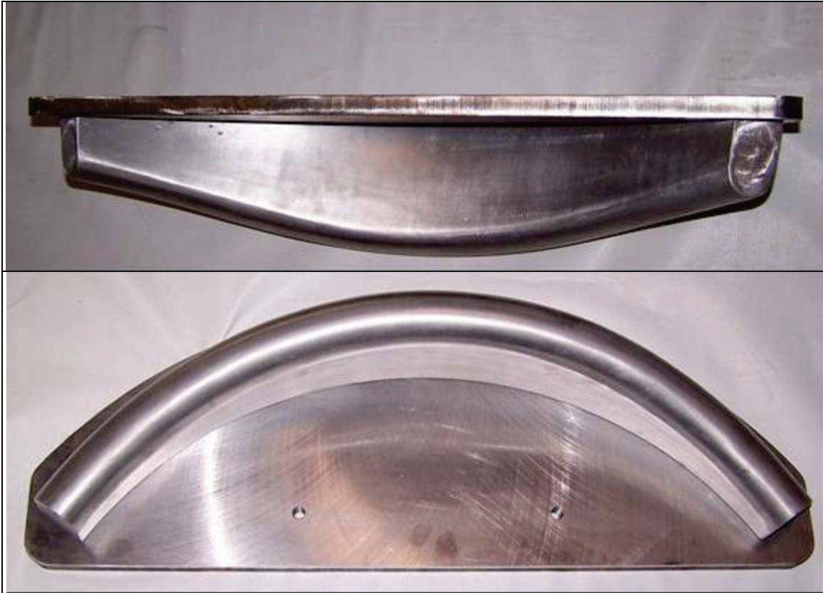
Figure 2.8. Bead Unseating Block BFNT 2C
