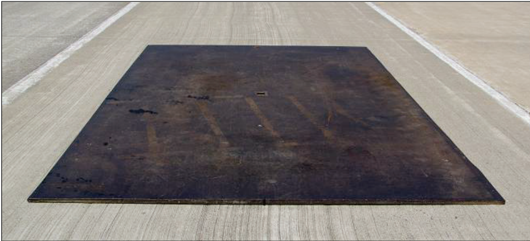
Figure 2.10. Steel Trench Plate Positioned on the TRC Skid Pad
