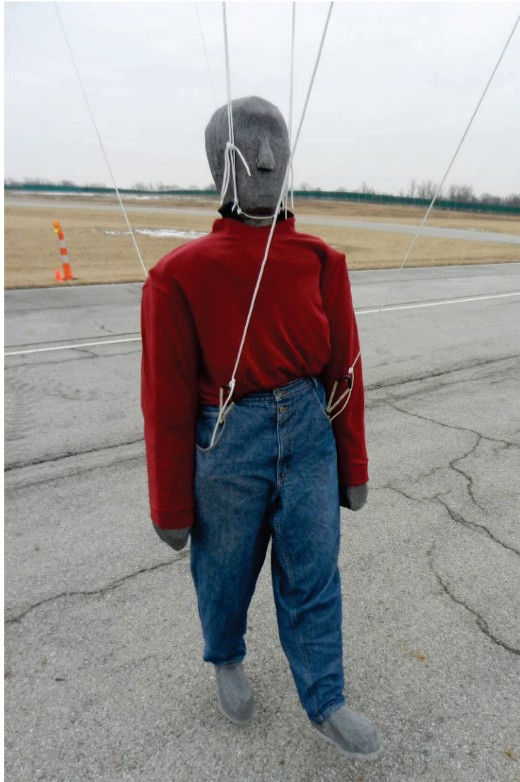
Figure 4: Adult Mannequin in Test Configuration
