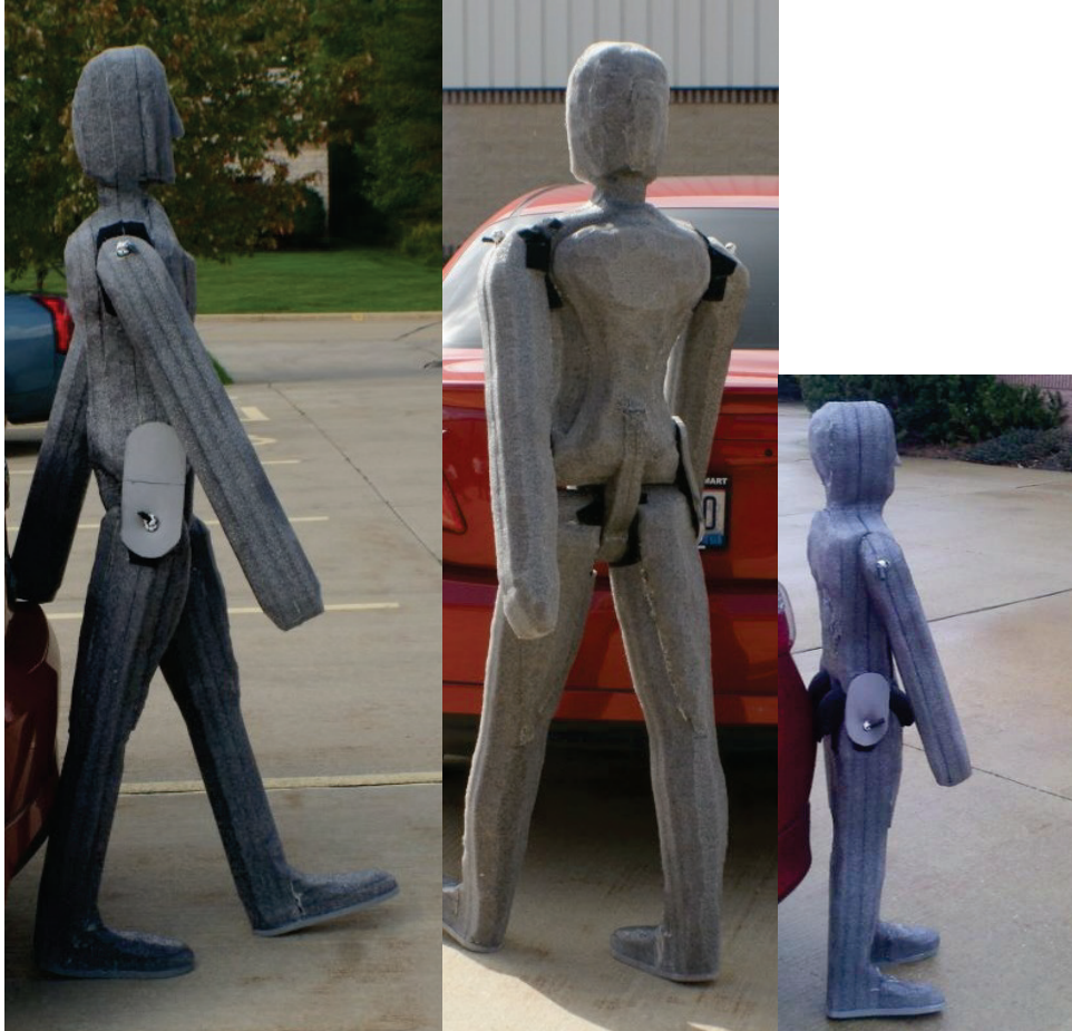
Figure 3: Illustrations of Pedestrian Mannequins: Adult Mannequin (Left and Center Photos) and 8-Year-Old Child Mannequin (Right Photo)
