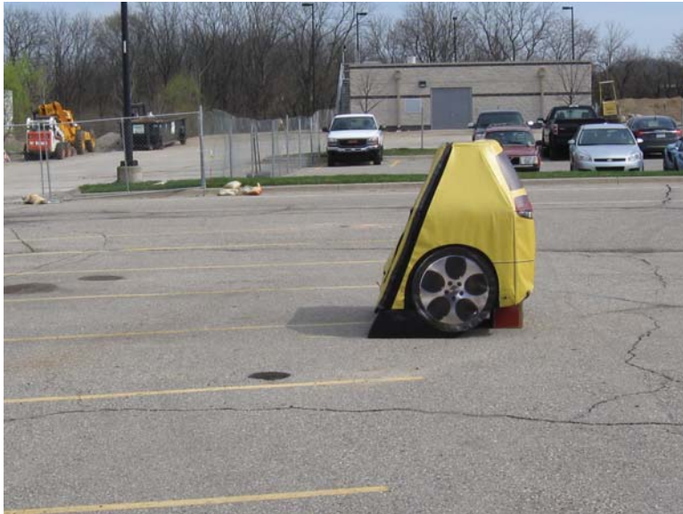
Figure 60: NHTSA Foam Car FC-2 Test Surrogate - Side View
