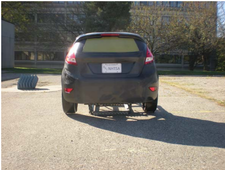
Figure 45: NHTSA SS_V2 Test Surrogate - Rear View.
