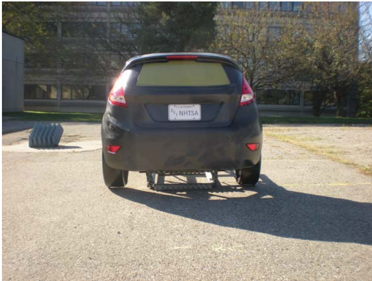
Figure 41: NHTSA SS_V1 Test Surrogate - Rear View
