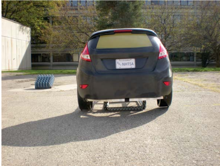
Figure 51: NHTSA SS_V2 Test Surrogate with metal band mounted under bumper.
