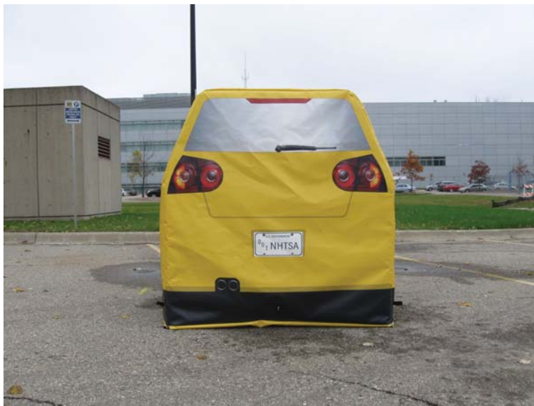
Figure 53: NHTSA Foam Car FC-1 Test Surrogate - Rear View
