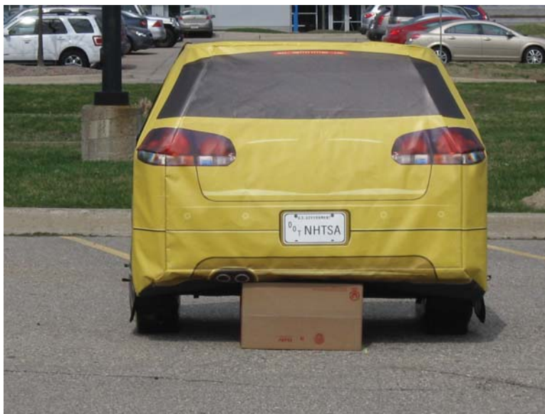
Figure 59: NHTSA Foam Car FC-2 Test Surrogate - Rear View
