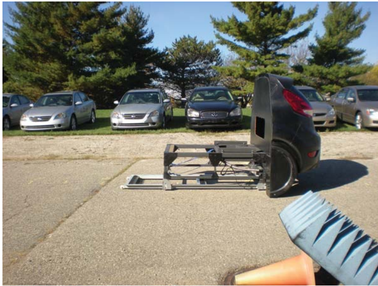
Figure 42: NHTSA SS_V1 Test Surrogate - Side View
