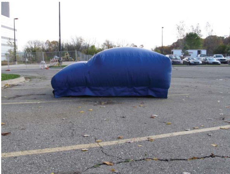
Figure 57: Helly-Hensen Balloon Test Surrogate - Side View
