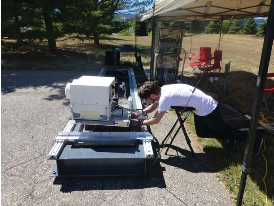
Figure 2: The W-band head is shown on the translation stage. A technician verifies the azimuth and elevation of the pan-tilt head.
