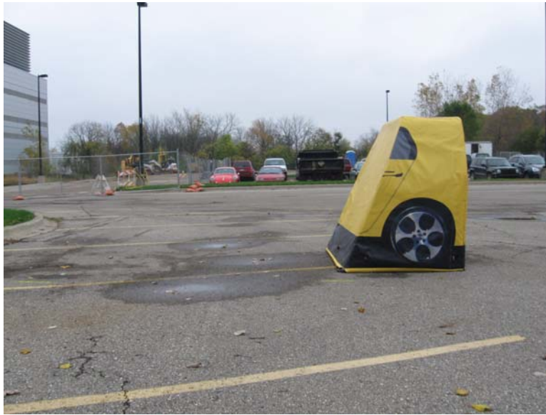
Figure 54: NHTSA Foam Car FC-1 Test Surrogate - Side View
