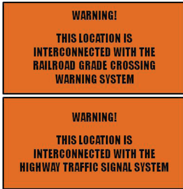
Figure 8: Example Warning Labels
