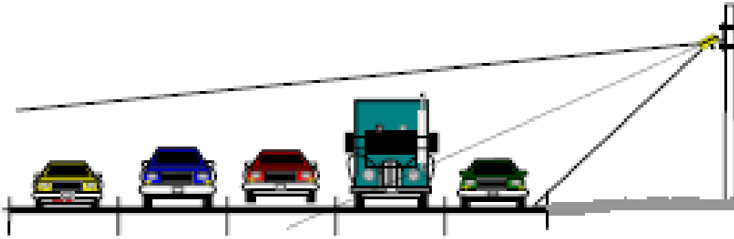
Figure 25. Side-mounted configuration of an FMCW microwave presence-detecting radar illustrating multilane vehicle detection. (Photograph courtesy of EIS, Toronto, Canada)
