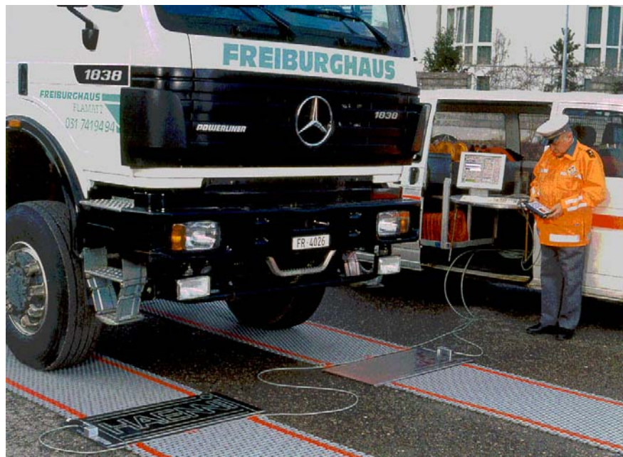
Figure 15. Capacitance mat sensor connected to data analysis equipment. (Photograph courtesy of LoadoMeter, Corp., Baltimore, MD).
