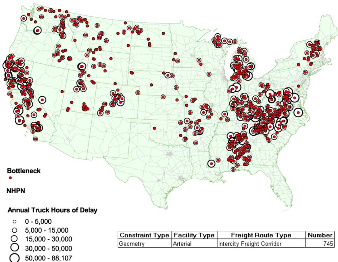
Figure 5.4 shows the distribution of truck hours of delay by bottleneck for *all steep-grade bottlenecks*. The vertical-axis scale has been adjusted downward to the highest delay value in the chart. The figure shows only those bottlenecks identified from the HPMS Sample database and therefore undercounts the actual number of these bottlenecks. The delay hours shown are the unexpanded estimates for the individual bottlenecks.
