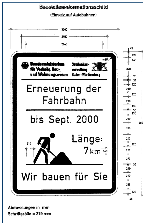
Figure 5. Sign prevalent in German work zones. “Renewing the Line until September 2000. Length 7 km. We Build for You.”
