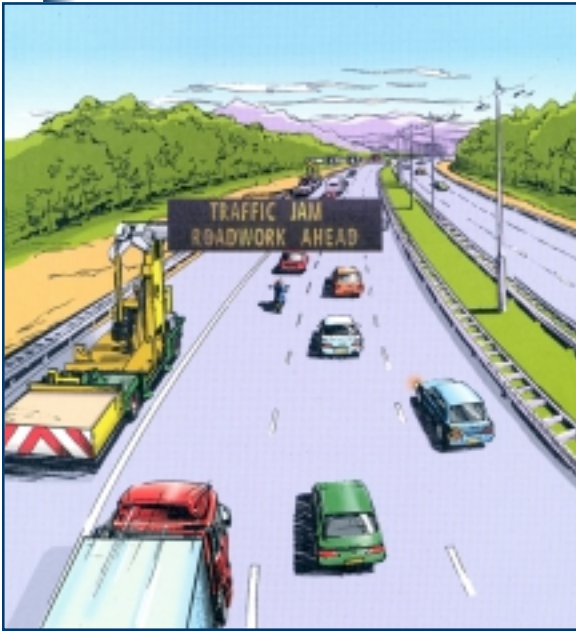
Figure 7. Currently 24 Mobile Lane Signalling Systems (MRS) are in use in the Netherlands, where they are installed as needed to warn motorists of work zones.
