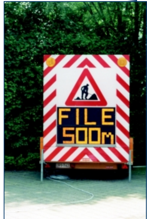
Figure 8. Trailer-mounted variable message signs are linked to video cameras in Belgium; as traffic slowdowns are detected, a warning is posted on the sign.
