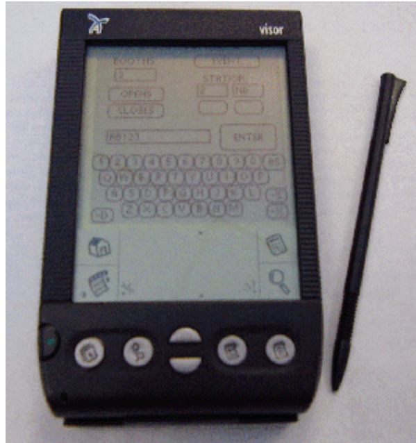
Figure 7. Data Collection Device and Software Application
