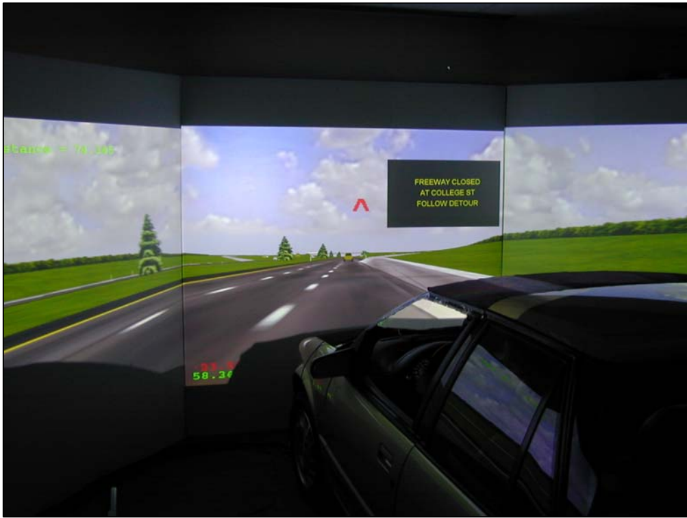
Figure 3. Another Image of the Simulated Driving Scene. Note the Message Display and the “Fall-Behind” Warning on the Screen.
