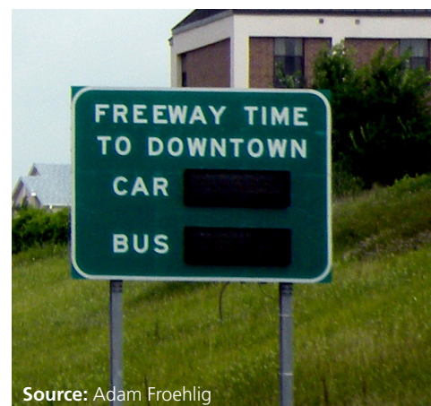
Figure 41. Photo. Signs displaying travel times via private vehicle and public transit can encourage modal shift during incidents.
