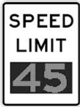
Figure 18. Illustration. MUTCD sign showing variable speed limits.
