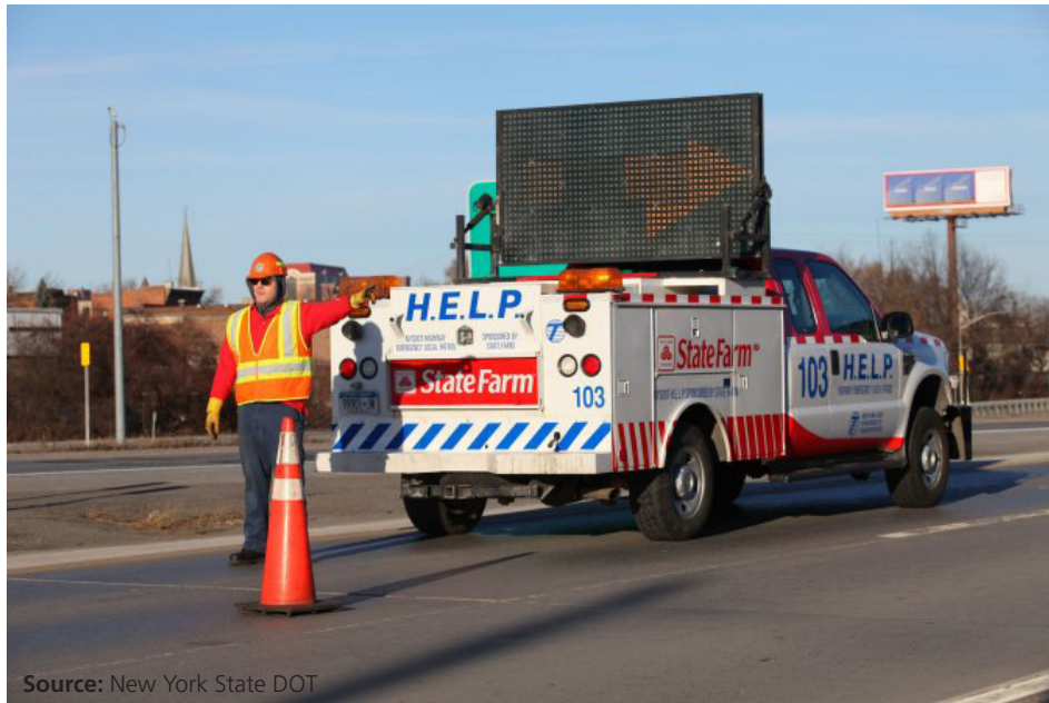
Figure 32. Photo. These New York State DOT HELP trucks have onboard cameras linked to the TMC to provide realtime incident information.
