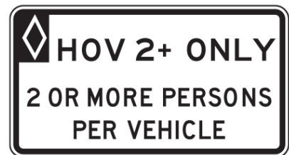
Figure 3. Illustration. MUTCD sign showing HOV lanes have a minimum vehicle occupancy requirement.
