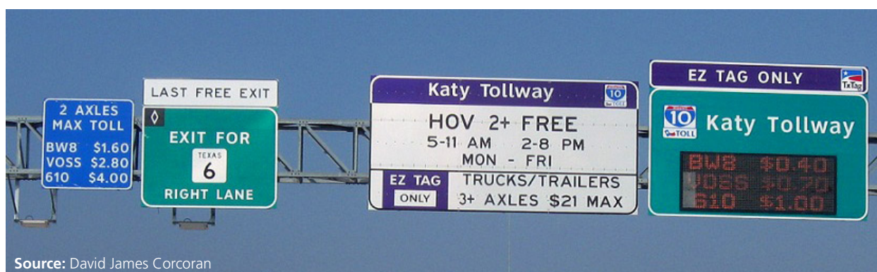
Figure 46. Photo. The Katy managed lanes (or Katy Tollway) operate as HOT during peak hours and ETL at other times, and have a maximum possible toll.
