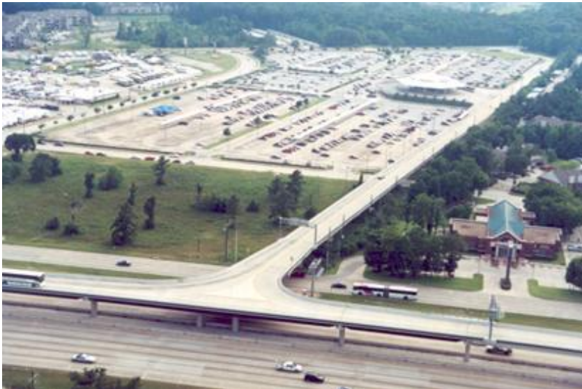
Figure 14: Direct Access Ramps to a Reversible Lane, Houston, Texas (courtesy of Texas Transportation Institute)
