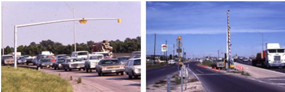
Figure 30: Junction (left) and Ramp Closure Controls (right)
