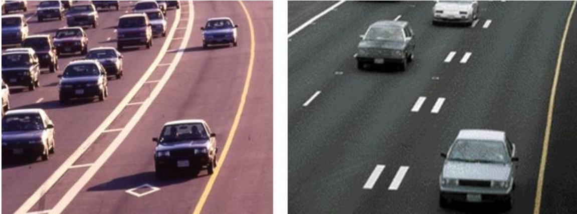
Figure 38: Examples of Buffer Separation Treatment
