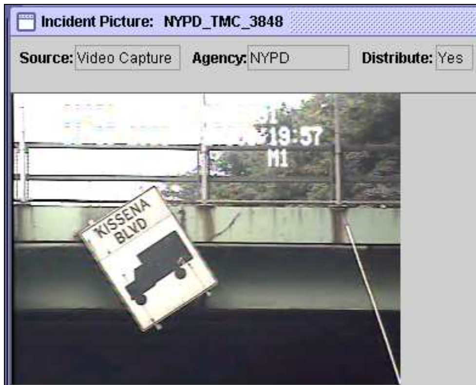
Figure 19. Unsecured Overhanging Sign in Incident 4886.
