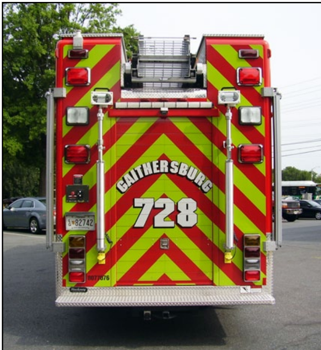
Figure 11—NFPA 1901-compliant fire apparatus chevrons.
