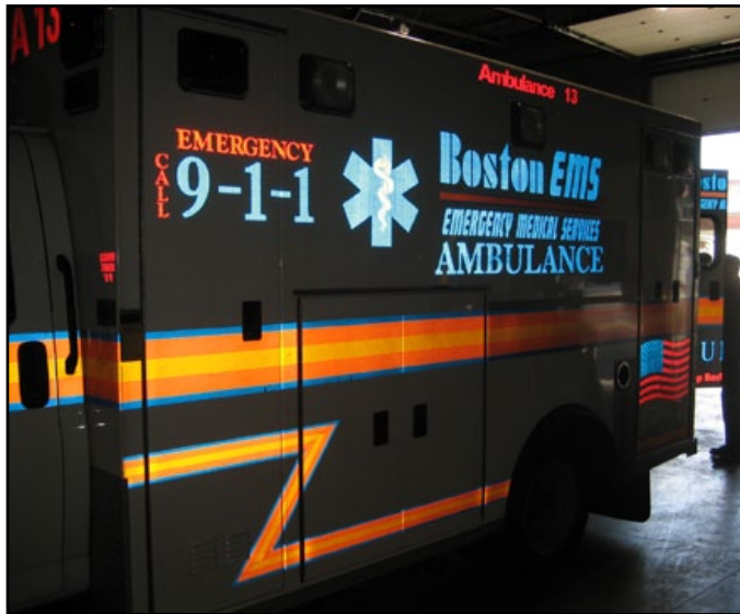
Figure 12—Retroreflective striping on GSA-compliant ambulance.
