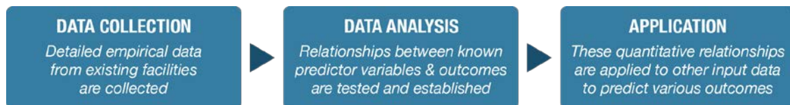
Figure 3. Flowchart. The general principle underlying typical HCM methods. (Source: Cambridge Systematics, Inc.)
