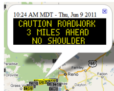
Figure 3-48. CMS Showing Road Work Message on Donner Pass in California from the One Stop Shop Google Maps™ Interface (Data Source: Caltrans, ODOT, WSDOT)
