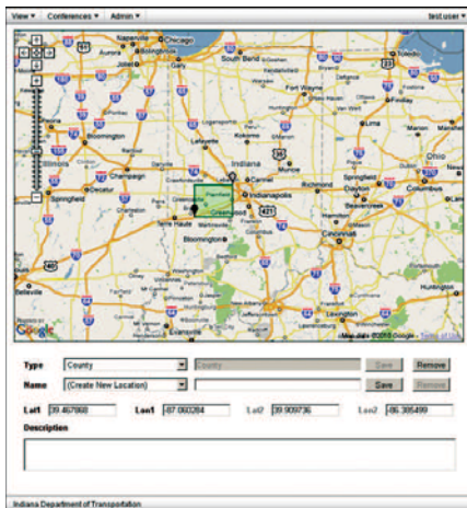
This screenshot from the Multistate Control Strategy Tool demonstrates how you can choose a location utilizing a bounding box and establish a location for future use. Courtesy of Mixon Hill, Inc.
