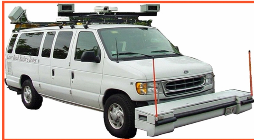
Figure 20. A typical van used to collect the video images. ( http://www.fhwa.dot.gov/publications/research/safety/05073/chapt2.cfm )
