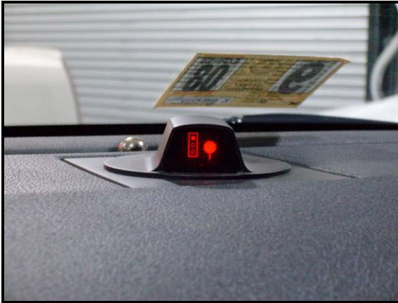
Figure 3 The visual display is located on the dash of the experimental vehicle.
