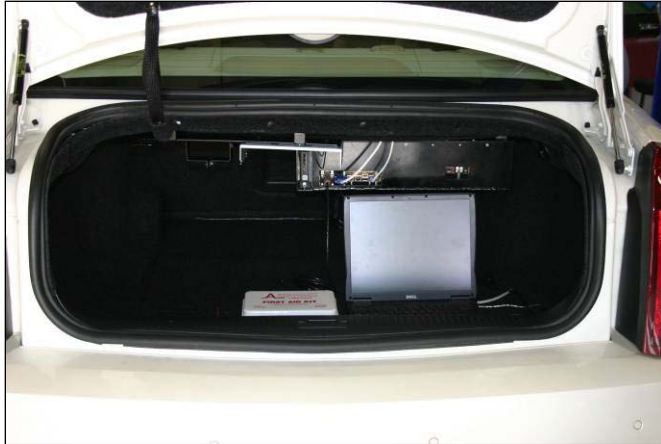
Figure 5 DAS, installed in the vehicle trunk underneath the rear shelf.
