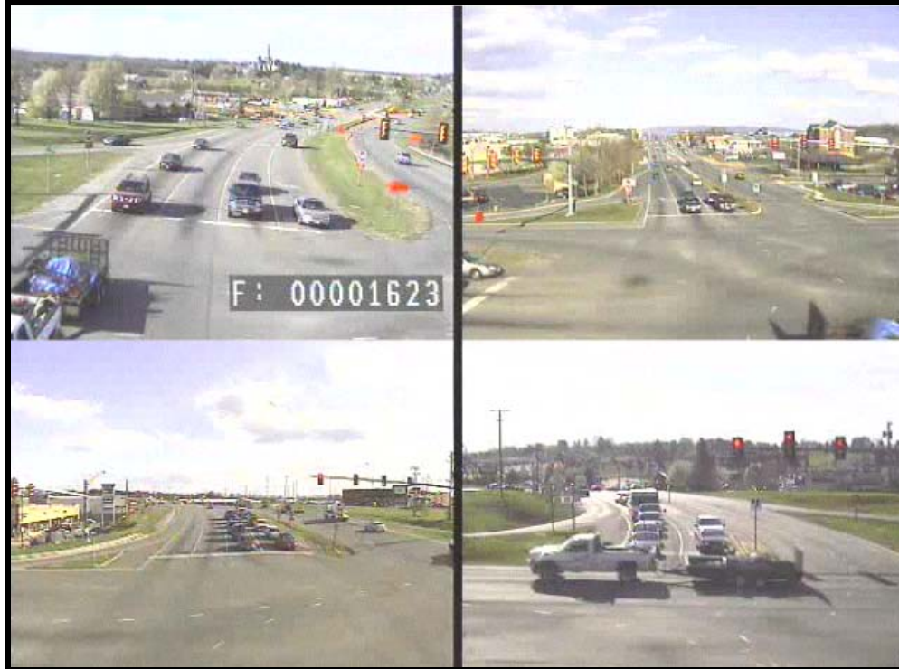
Figure 9 Video quadrants from camera units mounted on intersection mast arms.
