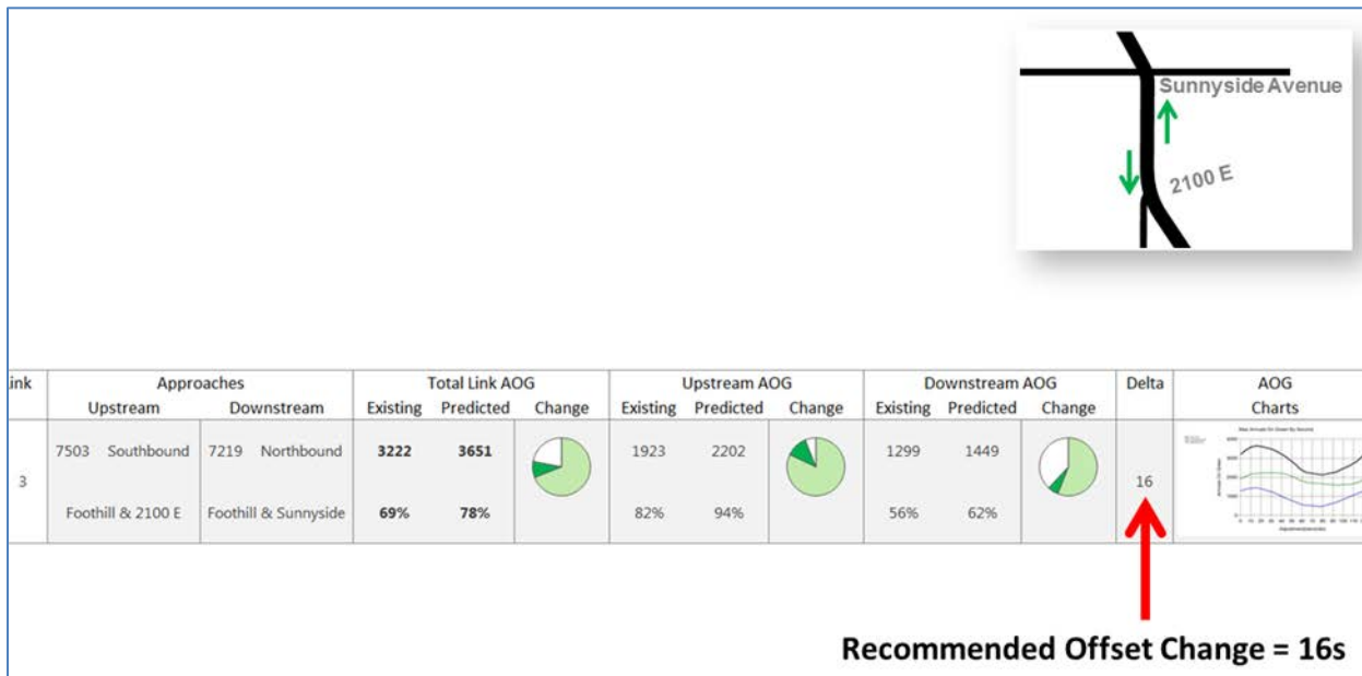
Figure 18. Graph. Using arrivals on green for optimization of offsets.
