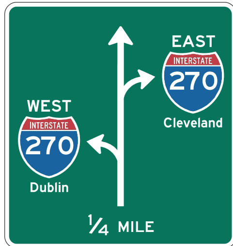
Figure 93. Ground-Mounted Diagrammatic Guide Sign for Urban Multilane Arterial, Used by Zwahlen et al. (2003)
