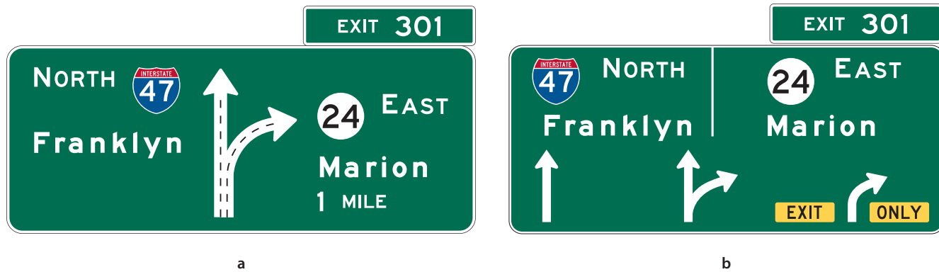
Figure 92. Example of MUTCD diagrammatic sign (a) and modified diagrammatic sign (b) used in comprehension evaluation (Brackett, Huchingson, Trout, and Womack (1992))
