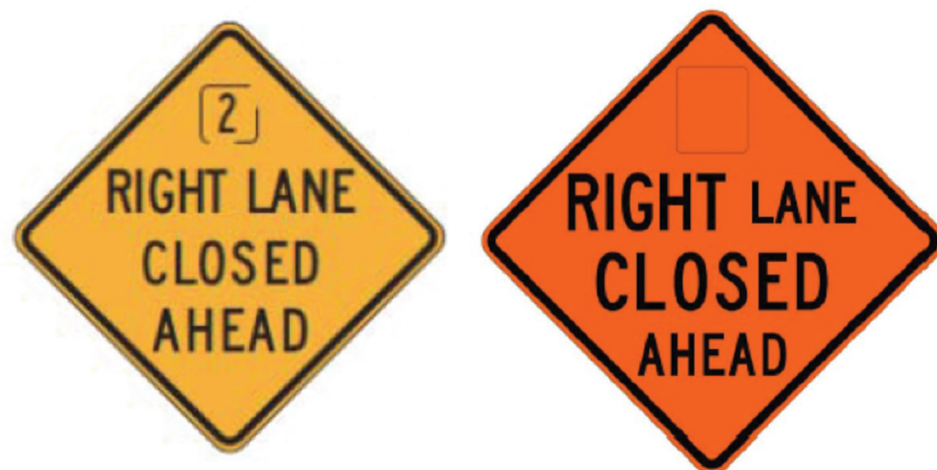
Figure 95. Current (left) and proposed modified (right) temporary work zone sign in California. (Caltrans 2012)
