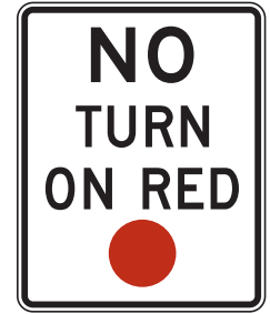
Figure 79. Novel Sign Tested as a Countermeasure to Reduce RTOR Violations and Pedestrian Conflicts (Zegeer and Cynecki, 1986)
