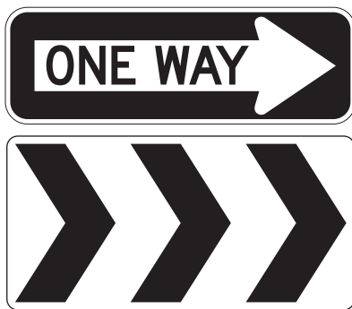
Figure 81. One Way and Chevron Sign Combination Used in Central Island of Roundabout (Jacquemart 1998)
