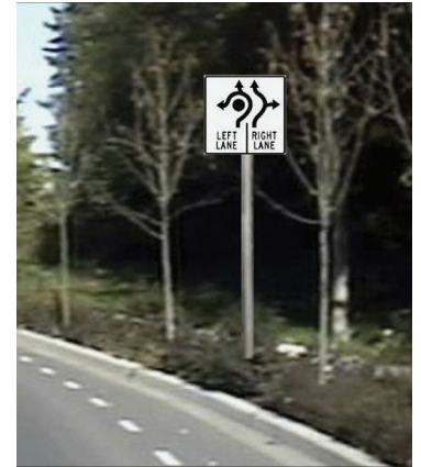
Figure 83. Lane Control Sign Recommended by Lord et al. (2007)
