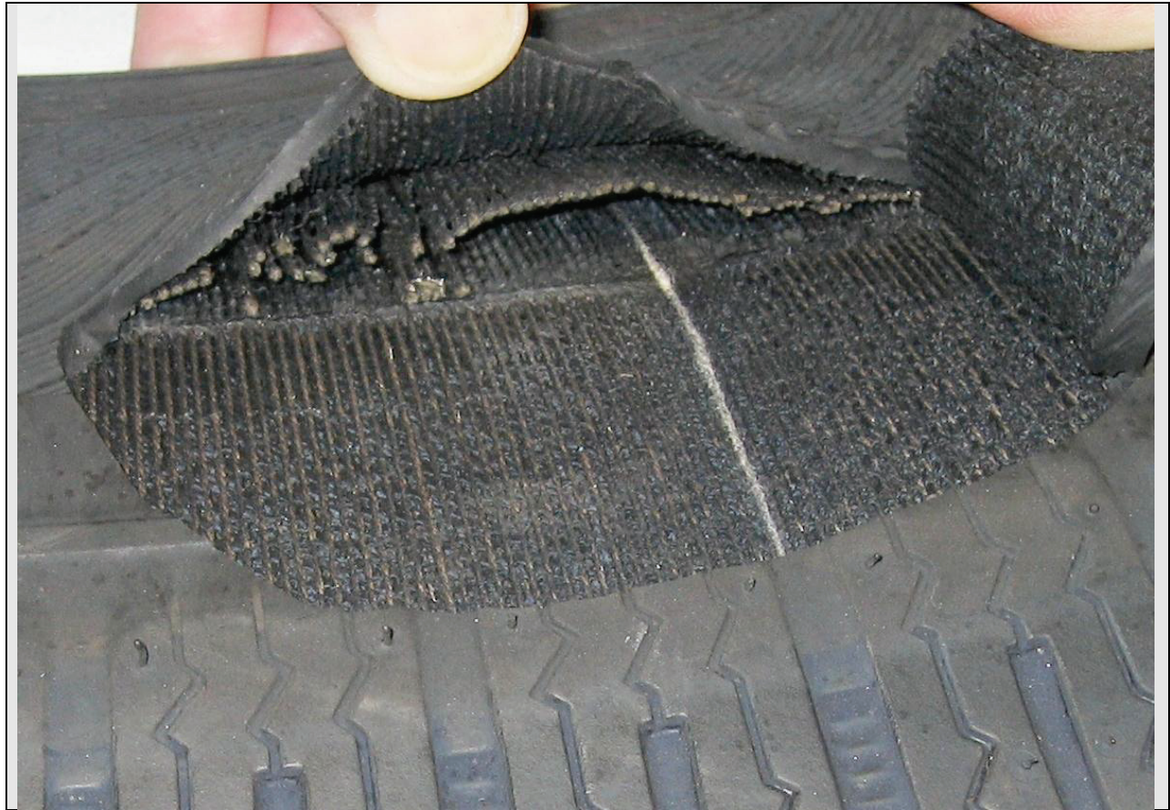
Figure 8. Failure at Ply End of Sidewall During Oven Aging
