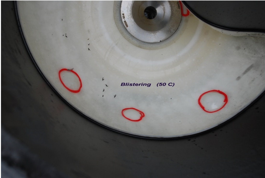
Figure 11. Red circles show blisters in the liner of the container that was cycled at +50°C.
