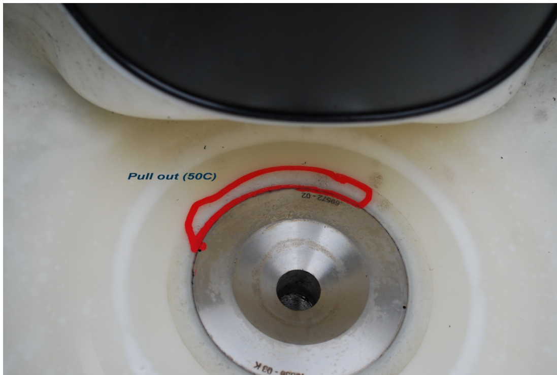
Figure 10. Interface between the liner and the boss of the container that was cycled at +50°C. The red shows where the liner pulled away from the boss.
