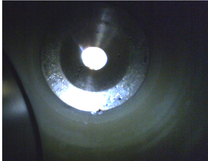
Figure 13. Container 1 (>30hr Hold Time) Following 500 Cycles and Two Time-at-Pressure Exposures.
