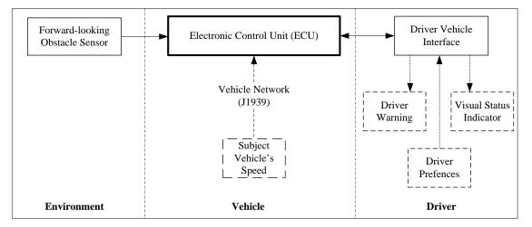
Figure 2. FCW System Architecture (Modified From ISO 15623: 2002)
