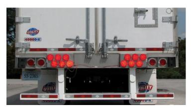
Figure 5. ERS Candidate System (Schaudt et al., 2010)
