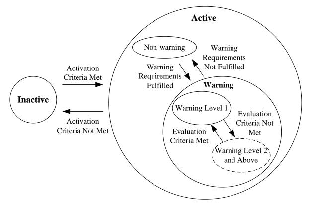
Figure 4. Side Collision Warning System Architecture (ISO 17387:2008)
