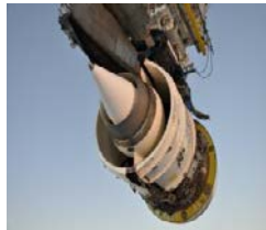
Boeing Ceramic Matrix Composite Nozzle Ground Test (TRL 6)
