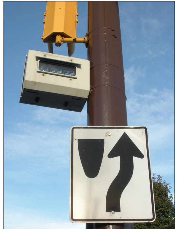
Figure 1: Red-light camera mounted on a signal pole
