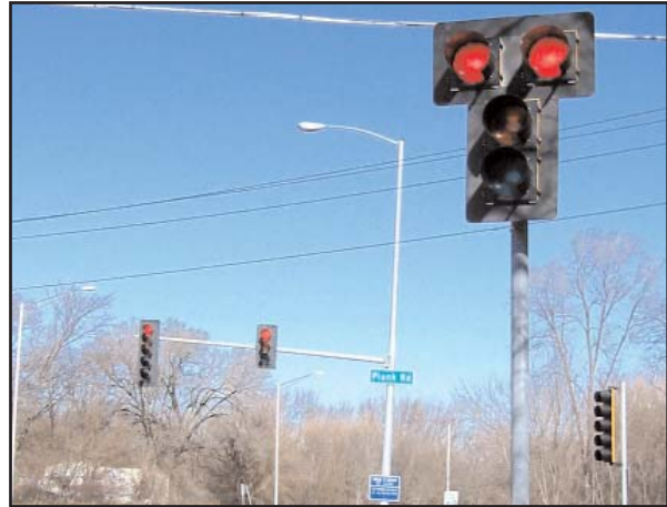
Figure 3–14. Field Use of Two Red-Signal Sections.
