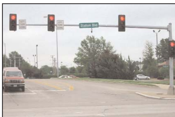
Figure 3–21. LEFT-TURN SIGNAL Signs at an Intersection.
