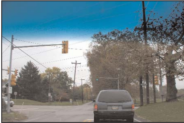
Figure 3–2. Post-Mounted Signal Blocked by Vehicle.
