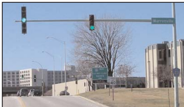
Figure 3-4. Intersection Approach with Two Signal Heads (Minimum).
