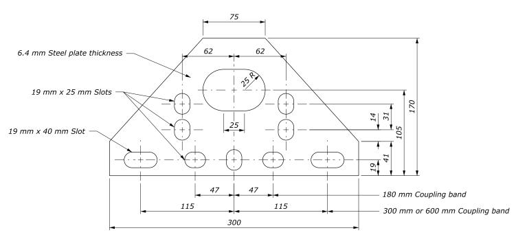
Measure length of coupling band parallel to the centerline of the pipe
